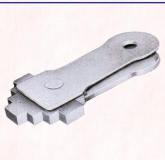
**HAMMERS:** Conventional hammers come with only one cutting edge. Premium Miracle mill has a unique design consisting of press-hardened steel maces which have several working edges. Hence the hammers have a working life several times more than the conventional hammers. Manganese steel hammers can be provided for tough materials.
