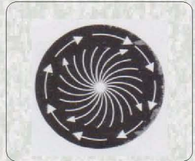
30° lead Average material will begin to spiral
