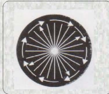
0° lead Average material will be thrown straight
