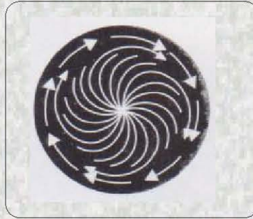
60° lead Average material will give maximum screening pattern
