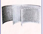
**SCREENS:** In Miracle Mill the Product is removed by the suction fan immediately after it is reduced to specified fineness. The degree of fineness is determined solely by the size of screens used. By changing the screen, material can be ground to the desired fineness. The screen can be changed in less than a minute.
