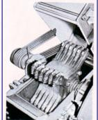
CLOSE UP OF HAMMERS AND MILL: The material is reduced to size on contact with a battery of hammers. The mill is self-protective. The hammers are hinged and fly backwards when foreign material accidentally enters the mill. There are four rows of hammers mounted on a shaft. The number of hammers in each row varies from model to model.
