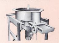
It is designed to discharge the material at required rate. Impeller is made out of C.I. or M.S. Casing made out of heavy duty plate. Outlet is provided with rack & pinion operated gate. Impeller is directly fixed on geared motor shaft, so overall it is very compact. Bottom is bolted construction for easy maintenance.
